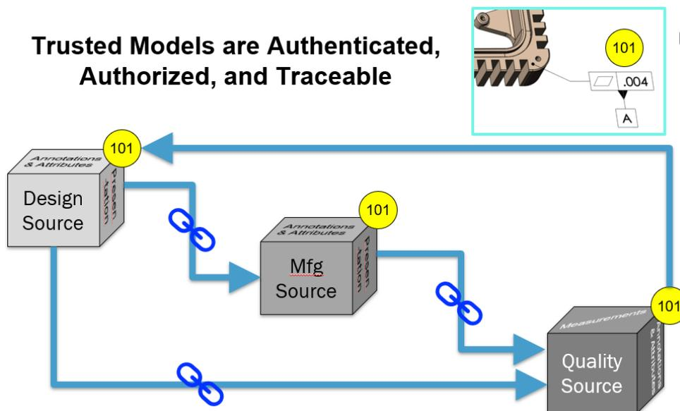
**Figure 3:** This pilot showed that data can pass from the Native NX Design Source to the SOLIDWORKS Manufacturing Source and record measurement results that can be viewed in 3D space (Quality Source). The 101 balloon is the unique identification that persists through all file formats.
